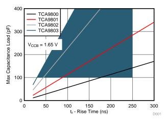
Figure 36. Selection Guide Based on Example Design Requirements for Bus C
