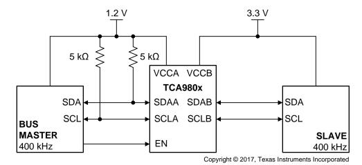
Figure 19. Typical Level-Shifting Application Example (Master on A-side)
