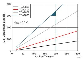
Figure 35. Selection Guide Based On Example Design Requirements for Bus B
