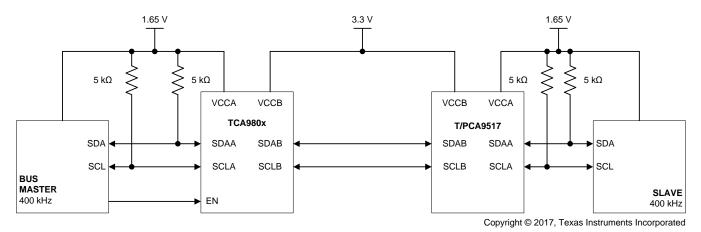
Figure 17. Incorrect B-Side Static Voltage Offset Buffer Connection
