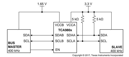
Figure 20. Typical Level-Shifting Application Example (Master on B-side)
