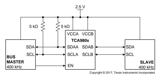
Figure 29. Buffering Use Case Without Level-Shifting
