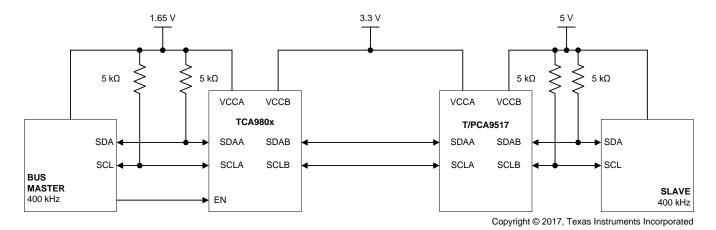
Figure 18. Correct Connection With Other Buffers
