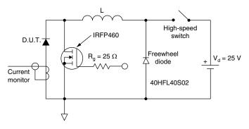
Fig. 8 - Unclamped Inductive Test Circuit
