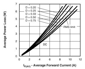
Fig. 6 - Forward Power Loss Characteristics
