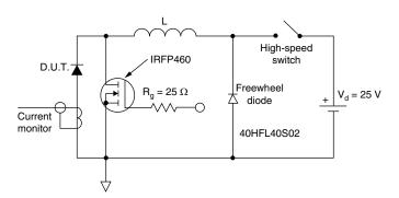
Fig. 8 - Unclamped Inductive Test Circuit
