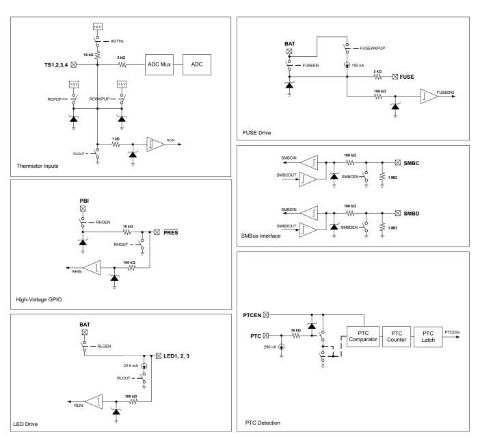
Figure 2. Pin Equivalent Diagram 2
