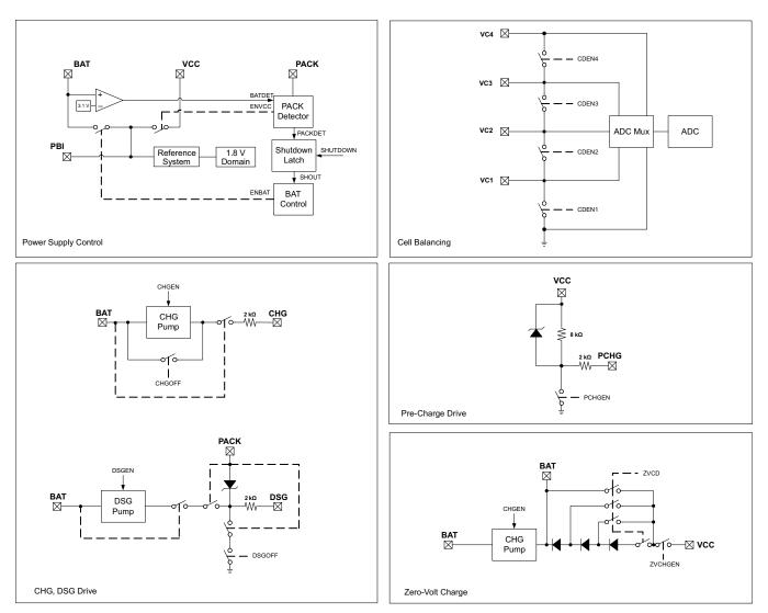
Figure 1. Pin Equivalent Diagram 1
