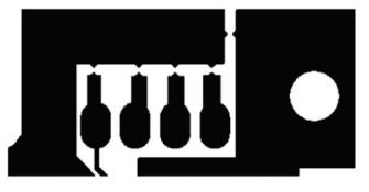
Figure 48. Recommended Spark-Gap Pattern Helps Protect Communication Lines from ESD
