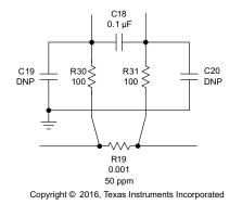
Figure 26. Differential Filter
