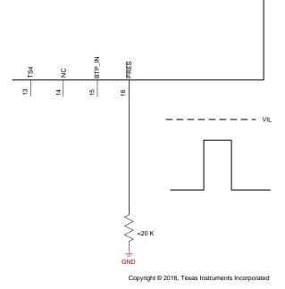
Figure 28. System Present Pull-Down Resistor
