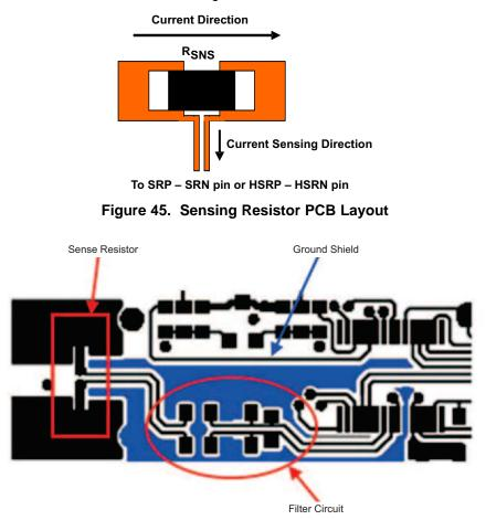
Figure 46. Sense Resistor, Ground Shield, and Filter Circuit Layout
