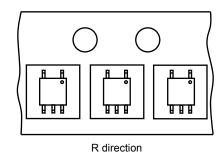
Figure 1 Device Orientation
