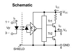
A bypass capacitor of  $0.1\mu F$  must be connected between pins 6 and 4.
