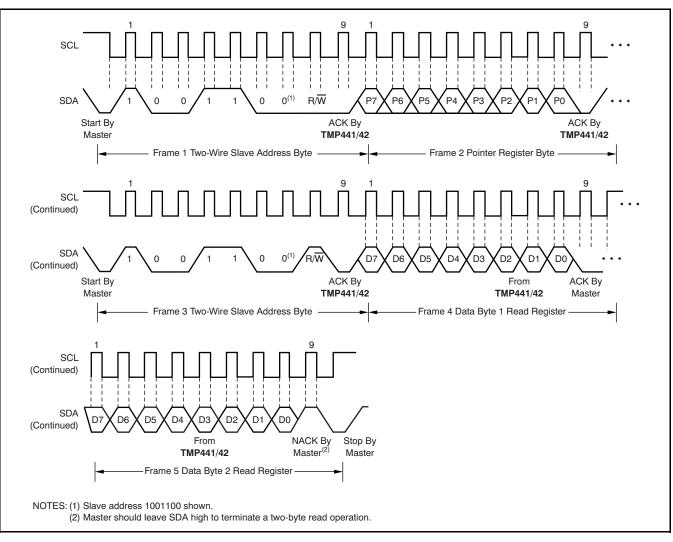
Figure 18. Two-Wire Timing Diagram for Two-Byte Read Format
