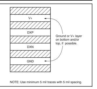
Figure 19. Suggested PCB Layer Cross-Section
