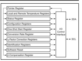
Figure 14. Internal Register Structure
