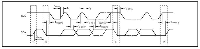
Figure 15. Two-Wire Timing Diagram
