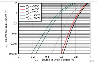
Figure 8. Normalized On-State Resistance vs Temperature Figure 9. Typical Diode Forward Voltage
