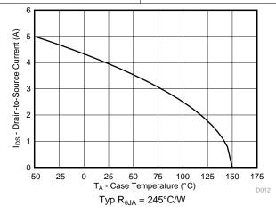
Figure 12. Maximum Drain Current vs Temperature
