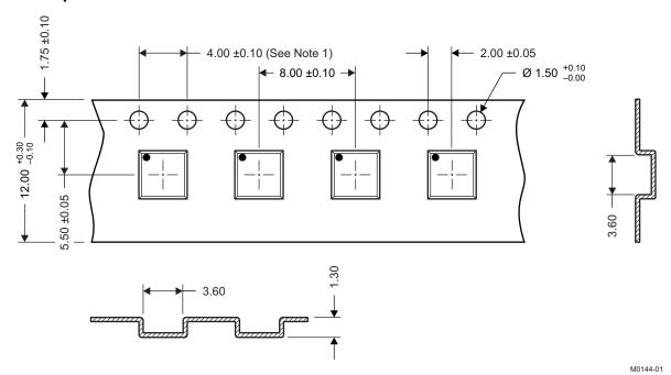
Notes: 1. 10-sprocket hole-pitch cumulative tolerance ±0.2
