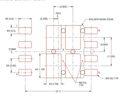
1. Laser cutting apertures with trapezoidal walls and rounded corners may offer better paste release. IPC-7525 may have alternate design recommendations.
