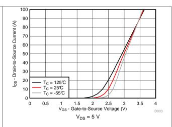
Figure 2. Saturation Characteristics
