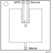
Max  $R_{\theta JA} = 60^{\circ} C/W$  when mounted on 1 inch² (6.45 cm²) of 2-oz. (0.071-mm thick) Cu.
