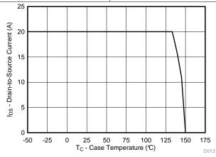
Figure 12. Maximum Drain Current vs Temperature
