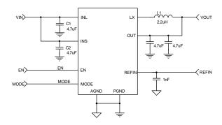
Figure 1. SKY87000-13 Typical Application Schematic
