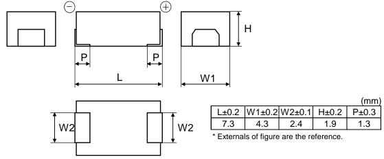
Surface finish of terminal : Tin(Sn) Material of terminal : Cu or Fe
