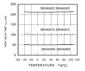
Fig.13 Output Delay Time "Low"→"High"
