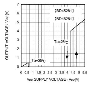
Fig.6 I/O Characteristics
