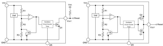
Fig.15 (BD45xxx Type Internal Block Diagram)
