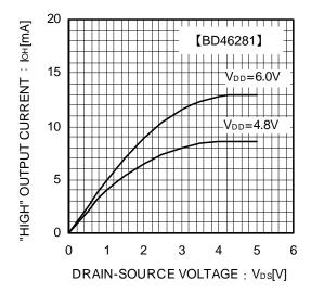
Fig.5 "High" Output Current
