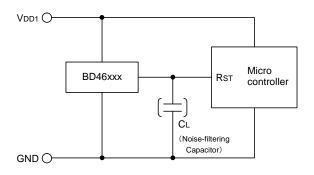
Fig.19 CMOS Output Type
