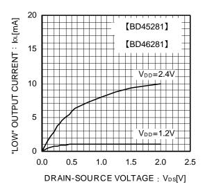
Fig.4 "Low" Output Current
