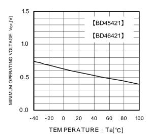
Fig.12 Operating Limit Voltage
