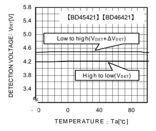
Fig.9 Detection Voltage Release Voltage
