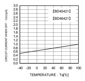
Fig.11 Circuit Current when OFF
