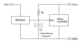
Fig.18 Open Drain Output Type
