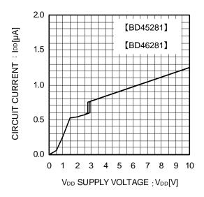
Fig.3 Circuit Current
