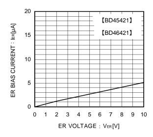
Fig.8 ER Terminal Input Current
