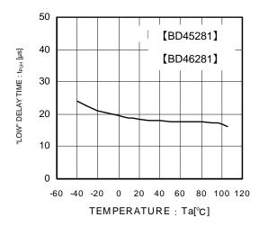
Fig.14 Output Delay Time "High"→"Low"
