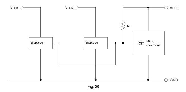
To reset the microcontroller when many independent power supplies are used in the system, OR connect an open drain output type (BD45xxx series) to the microcontroller's input with pull-up resistor to the supply voltage of the microcontroller (V<sub>DD3</sub>) as shown in Fig. 20. By pulling-up to V<sub>DD3</sub>, output "High" voltage of micro-controller power supply is possible.
