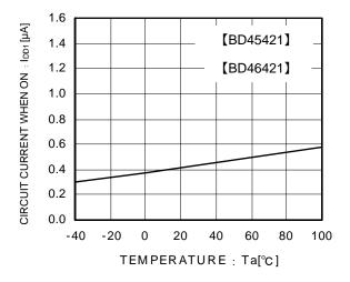
Fig.10 Circuit Current when ON (VDET-0.2V)
