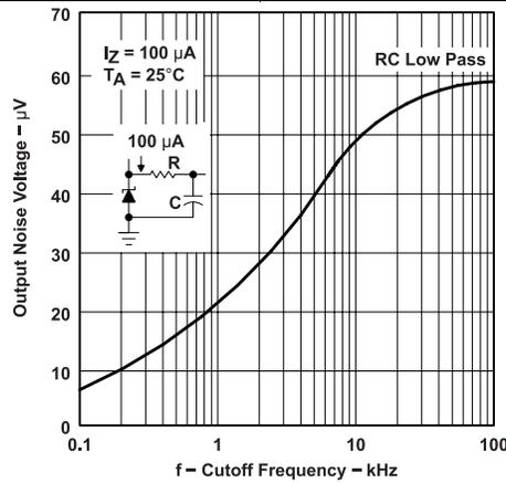
Figure 7. Output Noise Voltage vs Cutoff Frequency
