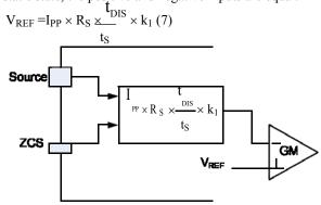
Fig.7 Output current detection diagram
