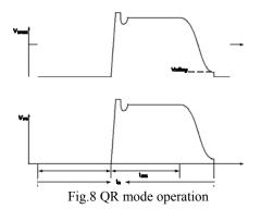
The voltage across drain and source of the primary integrated MOSFET is reflected by the auxiliary winding of the Flyback transformer. ZCS pin detects the voltage across the auxiliary winding by a resistor divider. When the voltage across drain and source of the primary integrated MOSFET is at voltage valley, the MOSFET would be tu ned on.
