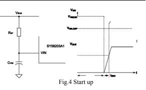
The start up resistor  $R_{ST}$  and  $C_{VIN}$  are designed by rules below:
